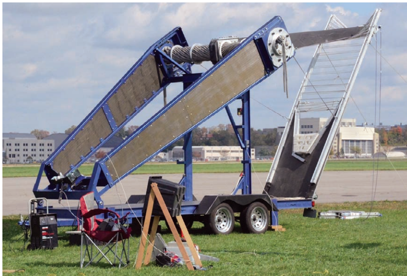
FIGURE 1. Torsion catapults use twisted rope to apply force to a swinging arm that hurls an object. Courtesy of John Camping, Team ETHOS.
