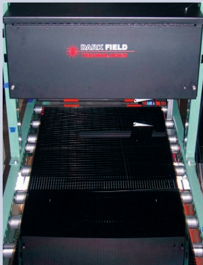
The Dark Field NxtGen Scribe 100 system inspects thin-film photovoltaic panels for scribe defects.
