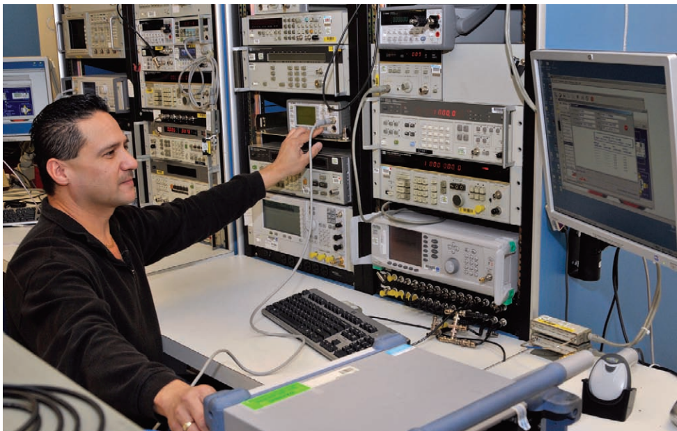
Technician Jerry Oppel calibrates spectrum analyzers on either of two automated stations.
